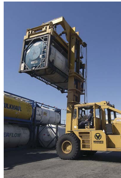
A special lift moves large tanks of liquid that are stacked on top of each other at the Ventura Transfer Company in Long Beach.
