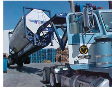
VTC built a custom hydraulic tractor that tilts the chassis to empty AES containers at Dial's manufacturing plant.
